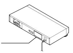
The rating plate and the safety caution are on the rear of the unit.
